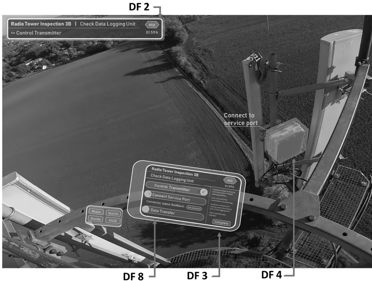
Figure 32. Reference HoloWFM user interface design for heads-up display, quick-access menu, and context-aware mode.
