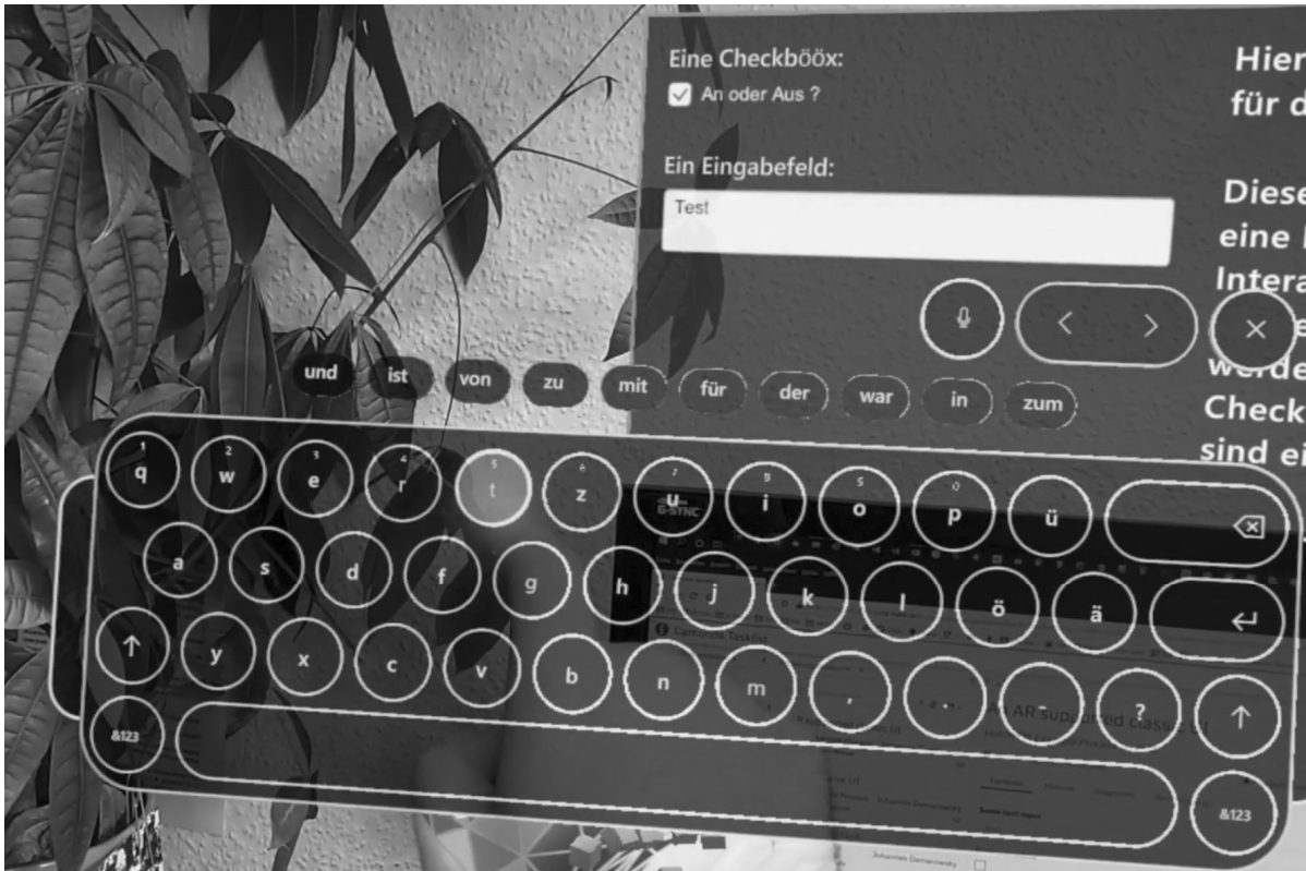
Figure 59. Screenshot from the HoloLens user's point-of-view of the virtual keyboard used to type in the input field.
